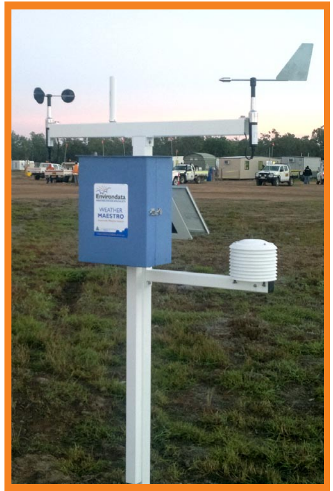
The Weather Maestro above is shown with the IS31 2m Mast, XA31 1m Cross Arm, LH35 Lockable Housing & MA30 Mounting Arm with SS31 Sensor Shelter
