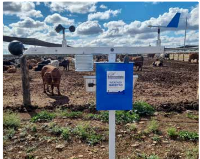
Feedlot Weather Station Weather Maestro installed 2025
