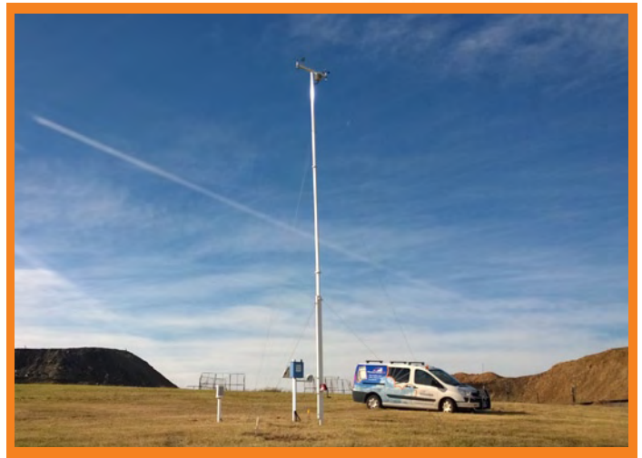
Full 10m Mast System Installed & Commissioned by Envirodata to meet Australian Standards
