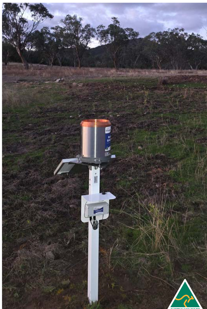
DS70 Remote Distributed Sensing Unit With RG50 Rain Gauge for remote rainfall monitoring
