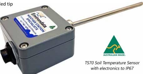
plane. An excavated access hole, and a 5mm drill bit to create the tip insertion hole in compacted soils may be required. (Tip diameter is 6.0mm)
