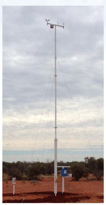
The 10m mast assembles from ground level, and winches into position, with no need for a crane or ultra-deep footings. It is able to be transported easily to site without the need for special lifting equipment. This allows for a single technician installation in truly remote sites.
