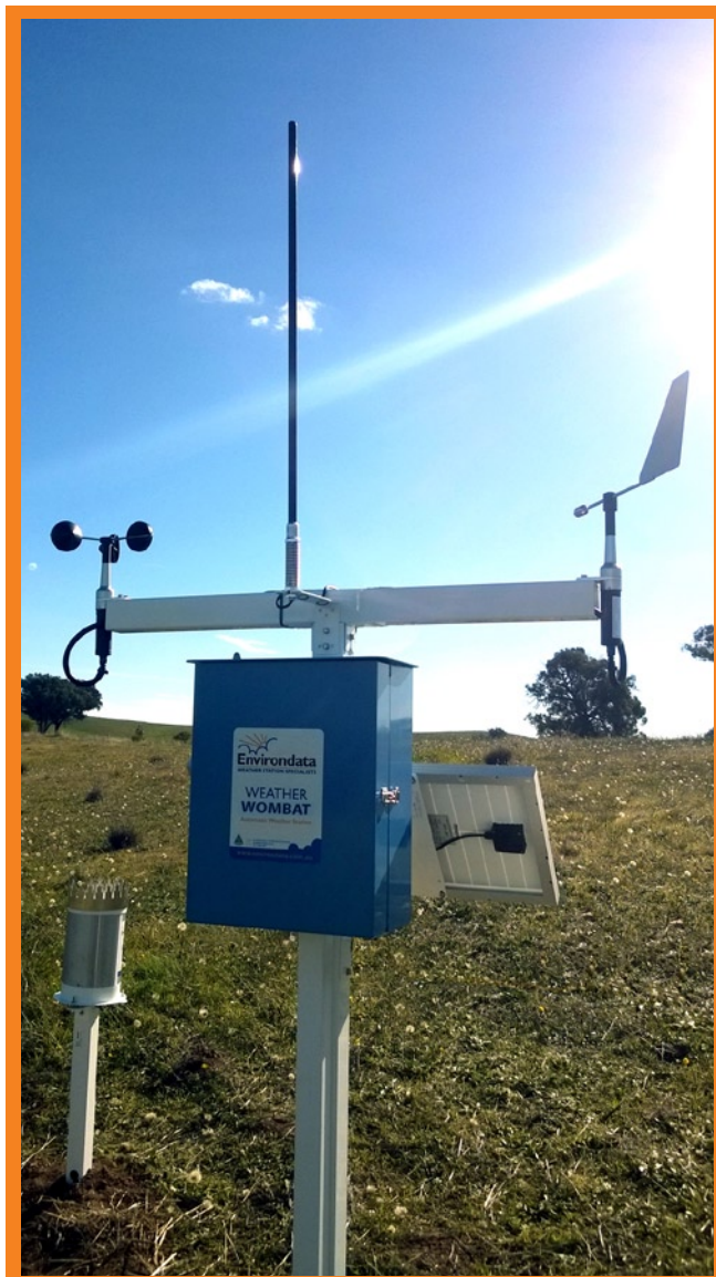
Weather Wombat in LH35 housing with wind speed, wind direction and rainfall sensors
