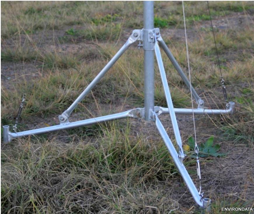
**3) Fit the tripod extension into the tripod base.**
