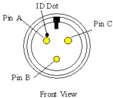
This is the view of the sensor connector mounted on the FA12 converter.
