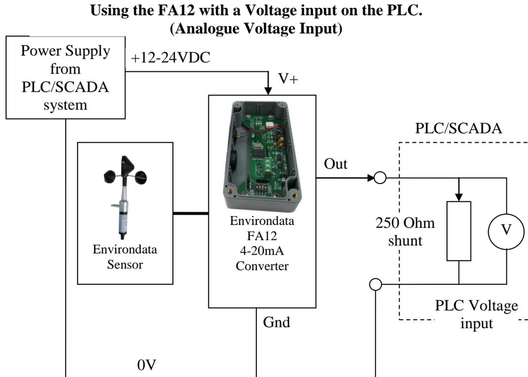
The FA12 can be connected to a Voltage input on a PLC. To do this, connect a 250 Ohm resistor across the Out and Gnd pins of the FA12. This will give a 1 to 5V signal range for 4 to 20 mA into the PLC.
