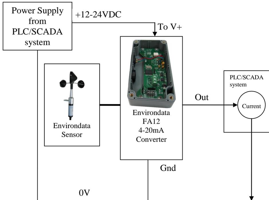
The FA12 4-20mA converter needs +Power, a GND path and the signal line connected. When connecting to a PLC or SCADA system, you must connect the signal out through the PLC and back via the 0V connection.
