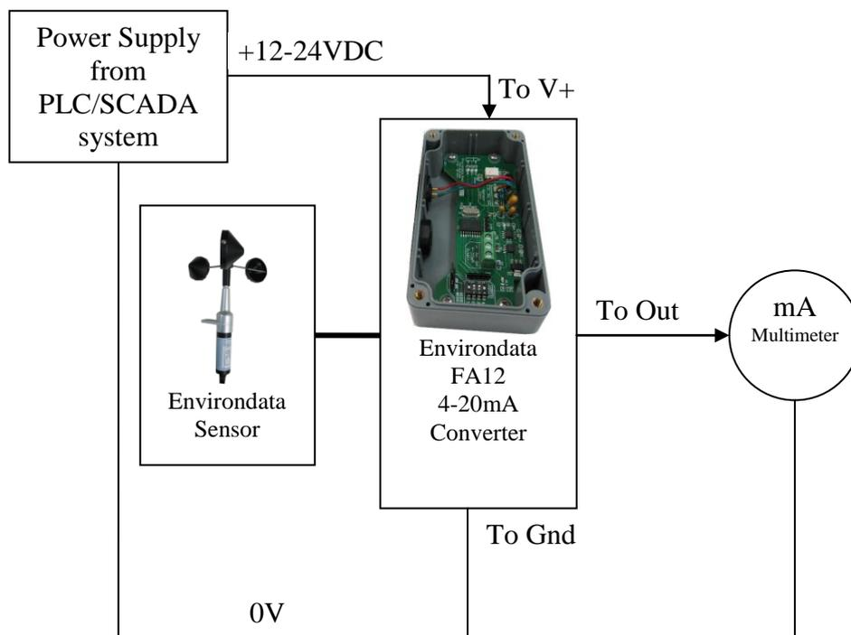
Connect a multimeter on its current setting and check the current values are as per the expected setup. (See Table1 in handbook).
