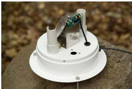
There should be clear ground for 2-3 metres around the rain gauge. The rain gauge should be mounted on a flat level surface, or a suitable mounting post with the top of the gauge perfectly horizontal.
