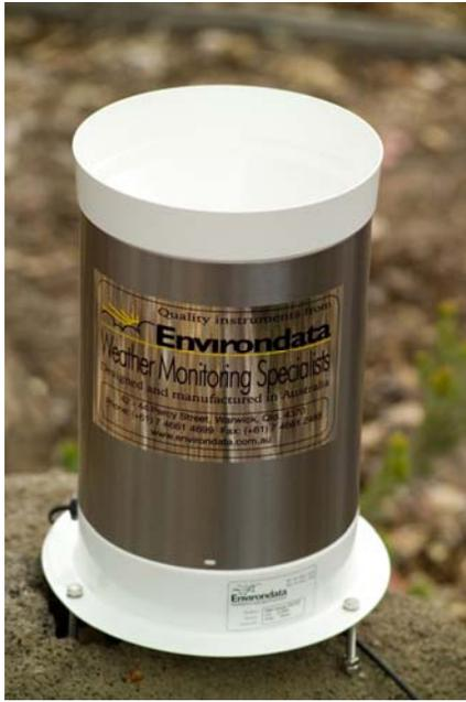
The rain gauge collects the rain in a standard 203 mm diameter funnel. It passes through a syphon and then collects in one of a pair of buckets arranged at each end of a tipping mechanism.
