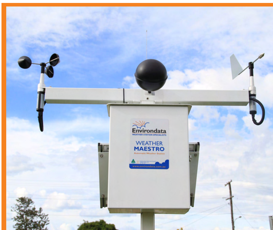
Weather Maestro Weather Station with BP40 installed in the cabinet to increase accuracy of vapour pressure and TWL calculations. Can also be used to calibrate on site scientific instruments
