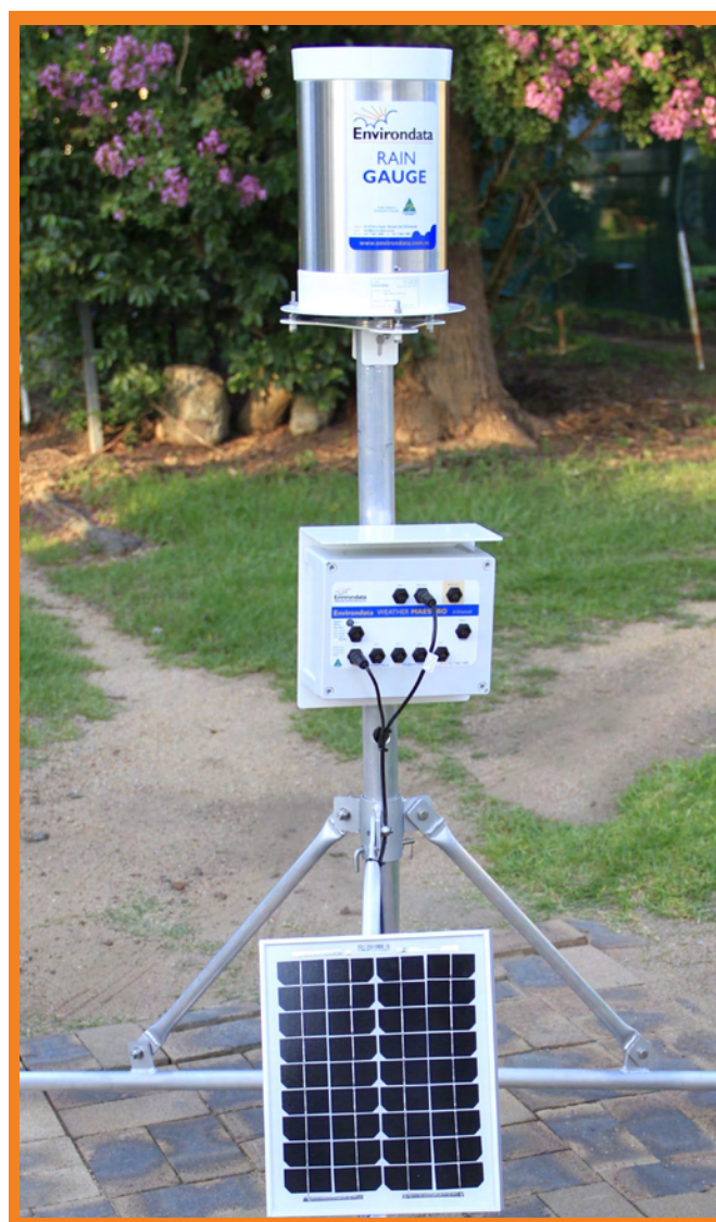
RG31 Shown includes tripod with solar panel for remote siting.
