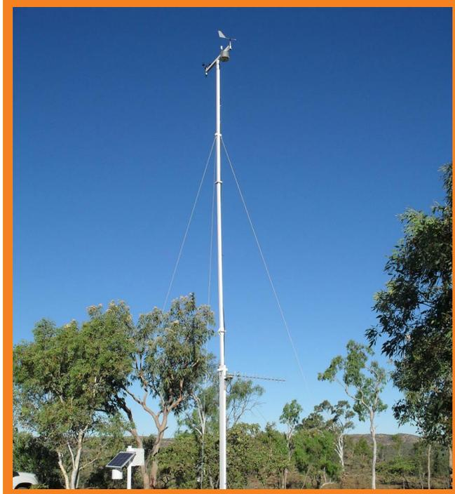
The Images above show two examples of Envirodata Weather Maestro weather stations with AD40 AirData firmware and ST30 Sigma Theta firmware loaded to simplify environmental reporting required at these mine sites. Both systems use our IS37 mast to meet Australian standards
